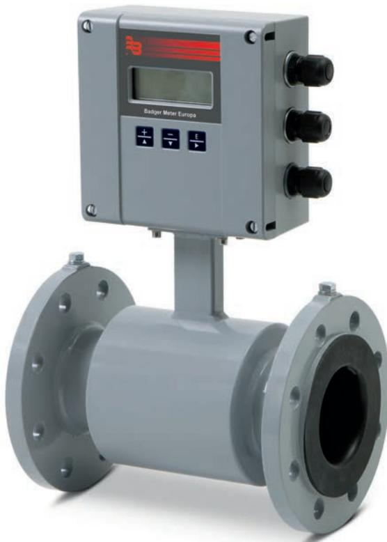
The amplifier type ModMAG® M2000 is best suited for bidirectional flow measurement of fluids with a conductivity  $> 5 \mu\text{S}/\text{cm}$  ( $> 20 \mu\text{S}/\text{cm}$  for demineralized water). ModMAG® M2000 shows a high accuracy, is easy to use and can be chosen for a large and flexible applications spectrum.
